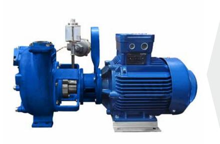
Suction port Threaded - 1 1/2" ISO 228 (BSP) Delivery port Threaded - 1 1/2" ISO 228 (BSP) Qmax 25 m<sup>3</sup>/h - 416 l/min (110 USgpm) Hmax 37 m (121 ft) Solids handling 11 mm (0.4") Motor power 4 kW - 5,5 HP Motor type **IEC** standard **Cast iron frame** Motor brand CEMP Weight 110 kg (243 lb)
